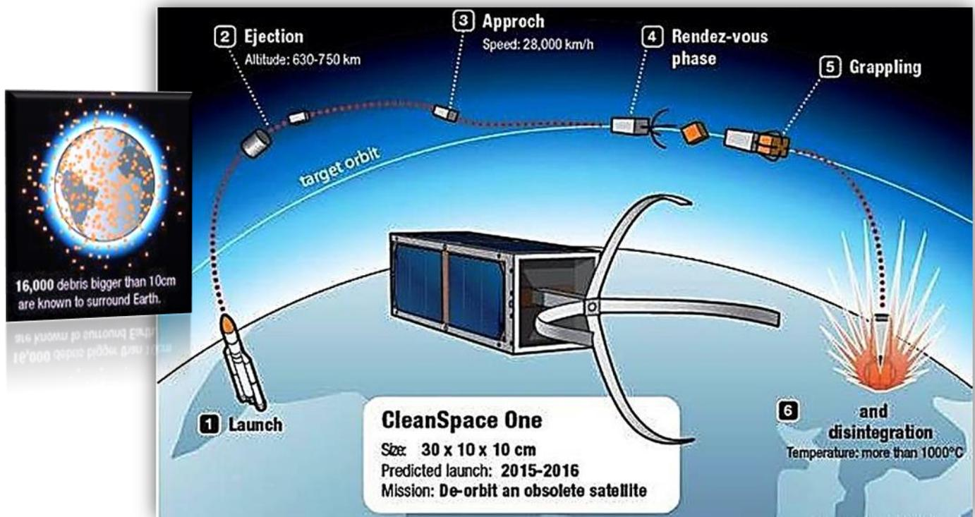
The proliferation of debris orbiting the Earth is an increasingly pressing problem for spacecraft. To combat this menace, the Swiss Space Center at EPFL is announcing today the launch of **CleanSpace One**, a project to develop and build the first installment of a family of satellites specially designed to clean up space debris.
